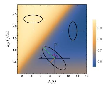
FIG. 1. Plot of the angle  $\theta/\pi$  at  $\gamma/\Omega=0.8$ . This angle is represented in the ellipse at the bottom of the picture. Here, the orange-solid (green-dashed) line represents the minor (major) axis of the Wigner function, i.e., that related to  $\delta_l$  ( $\delta_L$ ). The axes X and P are those of the phase space.
