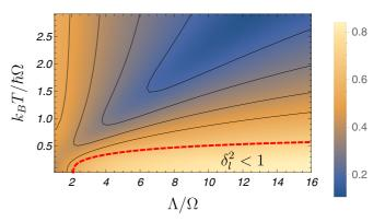
FIG. 2. Eccentricity of the Wigner function introduced in Eq. (28), at  $\gamma/\Omega = 0.8$ . The red dashed line represents the values of T and  $\Lambda$  yielding  $\delta_l^2 = 1$ , and we have genuine squeezing below it.
